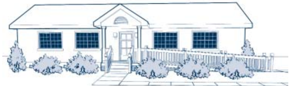
Plantings Minimize and Soften the Visual Impact of Ramps
